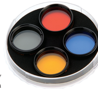
Celestron's Eyepiece Filter Set contains red, blue, and yellow filters that bring out details on the planets, and a neutral density filter for reducing the Moon's bright light. Celestron
