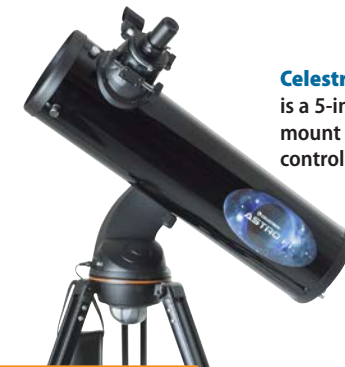
A reflector uses a curved mirror to focus light and a small, flat mirror to reflect it to the eyepiece. Astronomy: Roen Kelly, after Celestron
